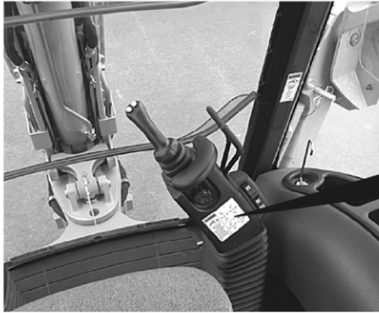
RIGHT BACKHOE CONTROL TOWER
